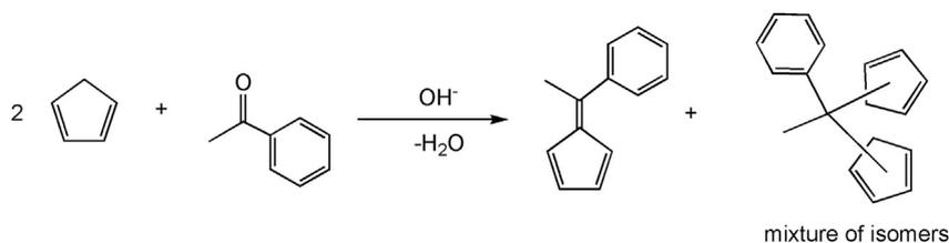
Scheme 1. Synthesis of the carbon-bridged bis-cyclopentadienyl ligand.
